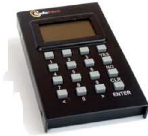
Figure 1 – Example of Trusted PIN Entry Device (Luna® PED II) that can be used with the TOE
